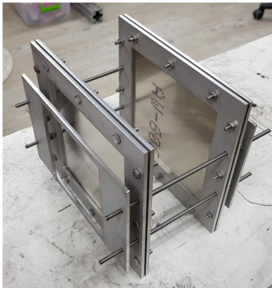
Fig. 1 Experimental jig with aluminum plate specimens
