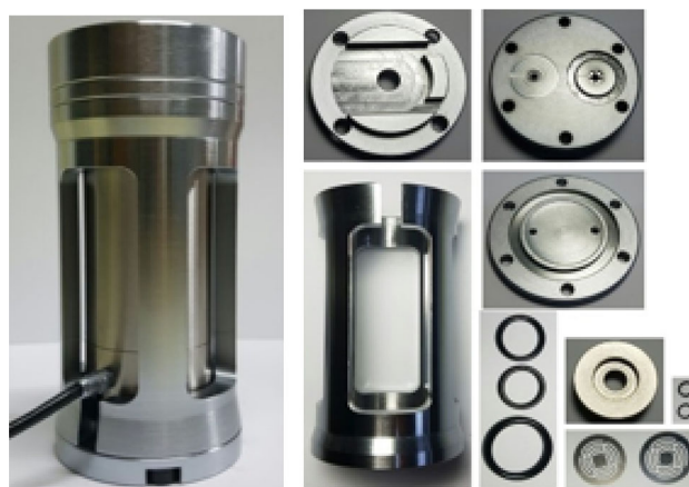
Fig. 13 Components of the designed piezoelectric-hydraulic pump
