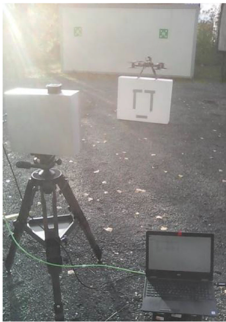
Fig. 6 Tracking scenario scene of two crossing drones using the MIMO-FMCW 8 × 16 radar system
