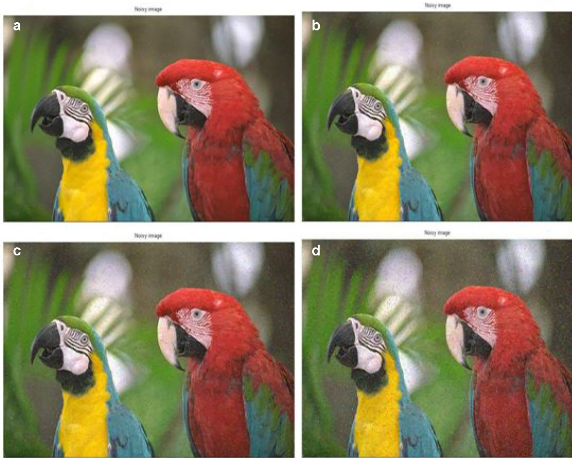
Fig. 3 a, b, c and d are the noisy images with noise probabilities 0.01, 0.03, 0.05 and 0.1 respectively
