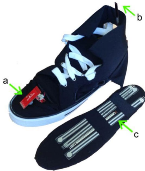
Fig. 3 Instrumented shoe. a Inertial measurement unit; b flexible goniometer; and c pressure sensors inside the insole. Adapted from Muro-de-la-Herran A, García-Zapirain B, Méndez-Zorrilla A. 2014 [16]
