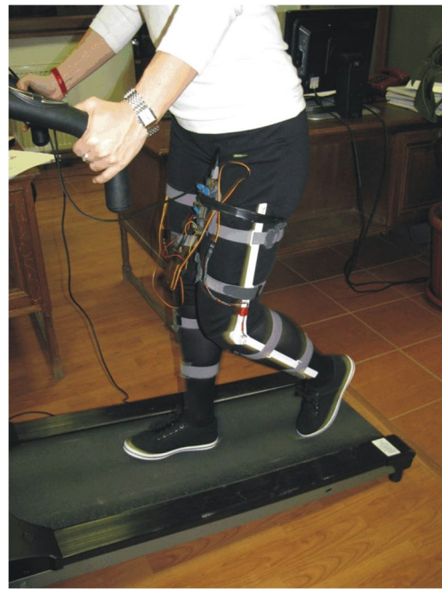
Fig. 2 Placement of electrogoniometers (strain gauge). Adapted from Tarniță D, Catană M, Tarniță DN. 2013 [31]
