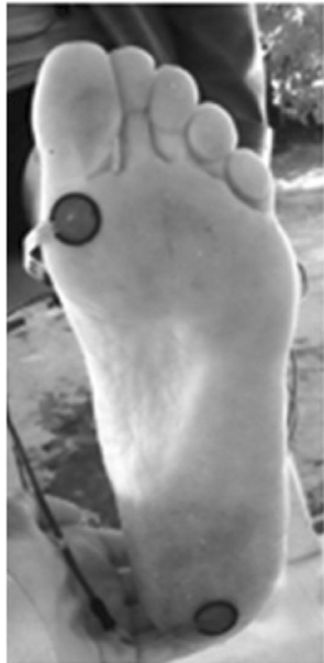
Fig. 4 Foot Switch (Noraxon®)—a pressure sensors positioning for gait assessment. Adapted from Spinoso DH, Bellei NC, Marques NR, Navega MT. 2018 [33]
