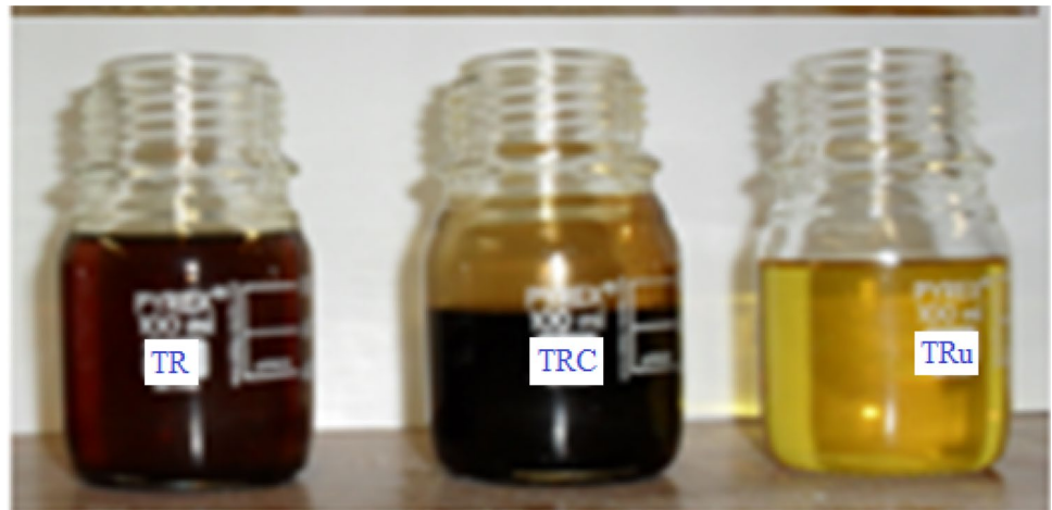
Fig. 3 Transformer Oils, TRu-Un-aged Transformer Oil, M-Thermally aged MIDEL7131 without copper, MC-Thermally aged MIDEL7131 with copper
