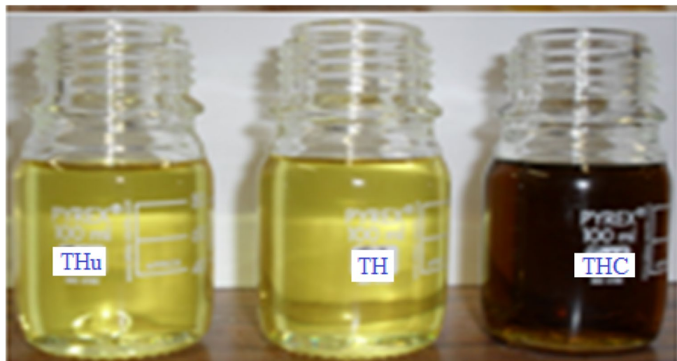
Fig. 4 THESO Oils, THu-Un-aged THESO Insulating Oil, Th-Thermally aged THESO without copper, THC-Thermally aged THESO with copper
