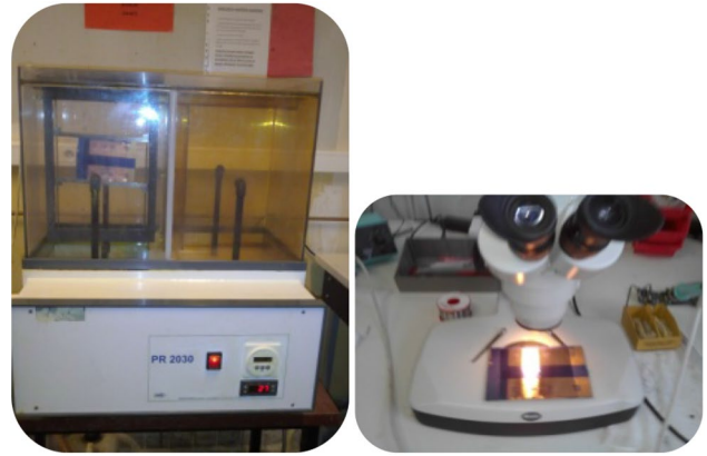
Fig. 10 System of chemical etching
