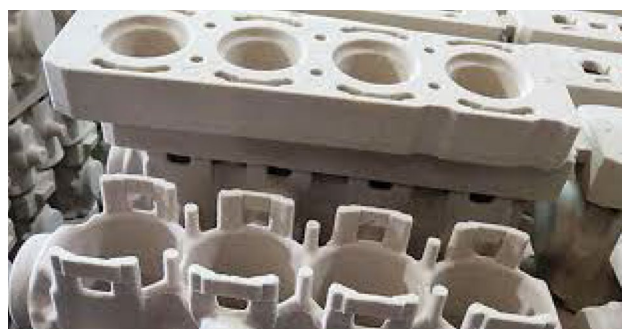
Fig. 11 Metal casting moulds from FURAN NO-BAKE process
