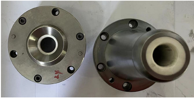
Fig. 29 Free bending dies with newly determined die structure parameters
