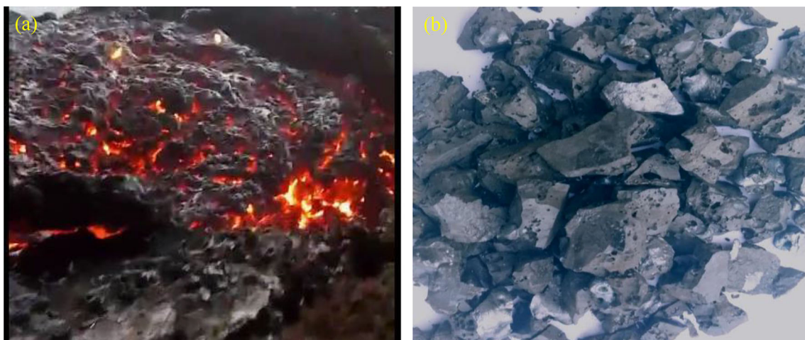
Fig. 1 Morphological characteristics of converter steel slag. a Hot steel slag; b cooled steel slag
