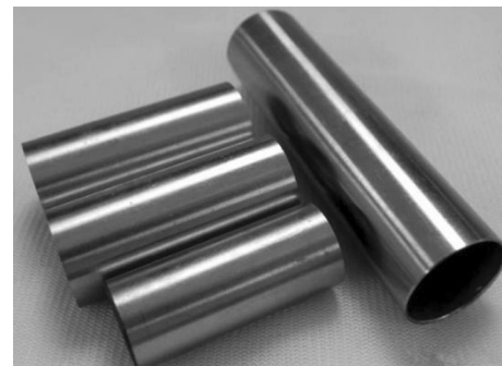
Fig. 10 Finished tube after rolling
