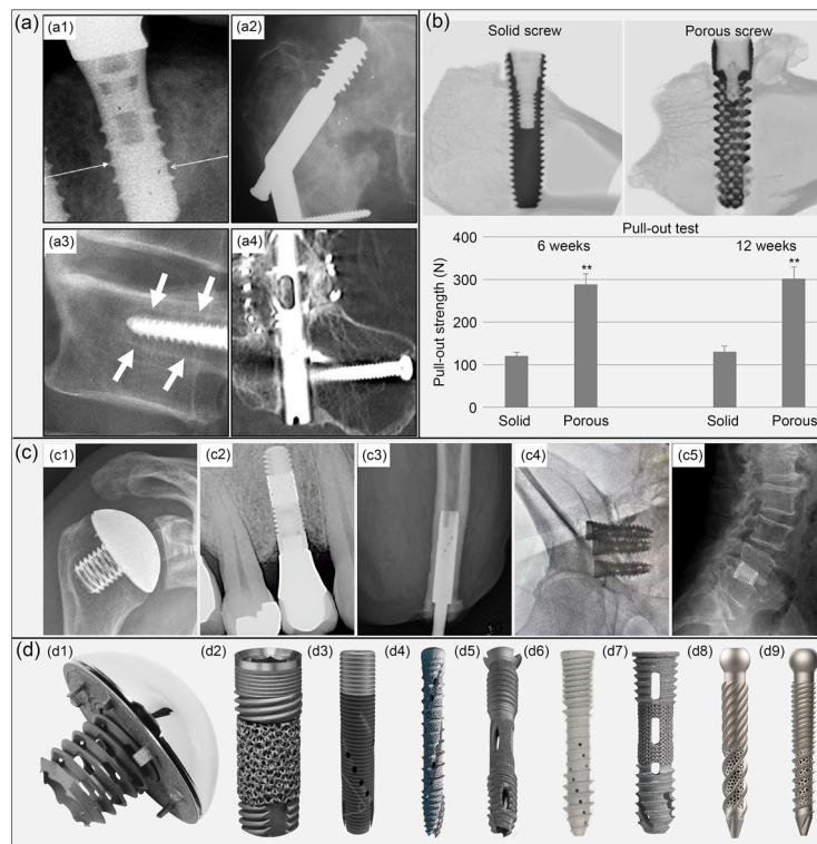
Fig. 2 Long-term loosening of conventional solid screws and existing porous screws. a Long-term loosening of conventional solid screws. a1 Decrease in height of the alveolar bone around the dental screw (Reproduced from [45], Copyright 2007, with permission from Wiley Periodicals, Inc.). a2 Lagging cutout of screw at femoral neck (Reproduced from [5], Copyright 2004, with permission from Lippincott Williams). a3 Peri-screw radiolucency in the vertebral body (Reproduced from [49], Copyright 2008, with permission from Lippincott Williams). a4 Peri-screw radiolucency in the calcaneus (Reproduced from [71], Copyright 2019, with permission from the authors, licensed under CC BY). b Comparison of micro-computed tomography analysis and pull-out test for solid screws and porous screws (Reproduced from [59], Copyright 2019, with permission from the authors, licensed under CC BY). c Radiographs of porous screws. c1 Radiograph of stemless total shoulder arthroplasty (Arthrex Inc., Naples, FL, USA) (Reproduced from [63], Copyright 2020, with permission from the authors, licensed under CC BY 4.0). c2 Radiograph of osseointegrated dental screws (Trabecular Metal Implants, Zimmer Dental Inc., California, USA) (Reproduced from [72], Copyright 2017, with permission from Allen Press Inc.). c3 Radiograph of the osseointegrated prostheses for the rehabilitation of amputees (OPRA, Integrum AB, Mölndal, Sweden) (Reproduced from [60], Copyright 2020, with permission from the authors, licensed under CC BY-NC-ND). c4 Radiograph of additive manufacturing (AM) osseointegrated screw for sacroiliac fusions (iFuse-TORQ, SI-BONE, California, USA) (Reproduced from [3], Copyright 2022, with permission from the authors, licensed under CC BY-NC). c5 Radiograph of porous screw cages (reproduced from [73], Copyright 2016, with permission from Korean Society of Spine Surgery). d Existing porous screws. d1 Photograph of stemless total shoulder arthroplasty systems (Arthrex Inc., Naples, FL, USA) (Reproduced from [62], Copyright 2018, with permission from the authors,
