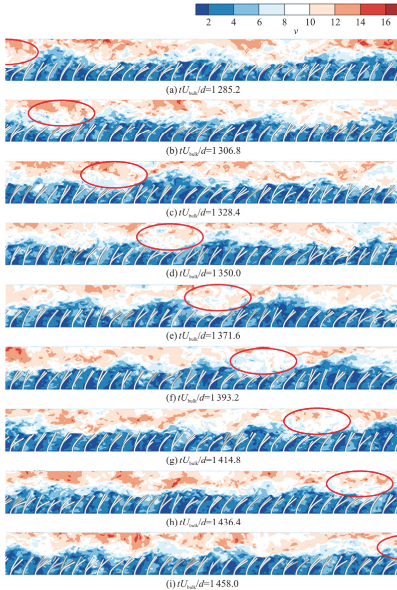
Fig. 18 (Color online) The instantaneous plant morphology and velocity distribution within the local area ( x/L = 0.25 - 0.75 ) of the vegetation (A2H1K2) (The positions of the same K-H vortex at different times are marked inside the red circle)
