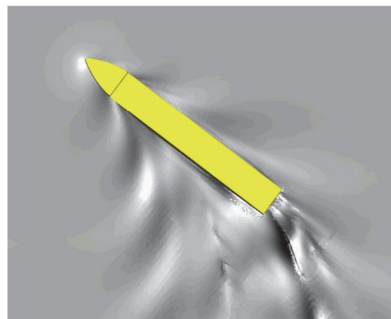
Fig. 16 (Color online) Free-surface distribution (TC-35 simulation, g3 )
