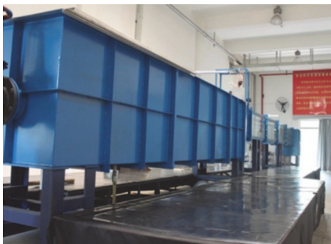
Fig. 7(a) (Color online) low Reynolds number recirculation water channel
