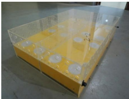
Fig. 3 (Color online) The perforated pontoon breakwater (Model 2)
