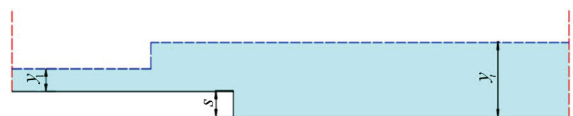
Fig. 3 (Color online) Schematic figure of the geometrical setup. Solid black lines indicates solid walls, dashed blue lines the initial free surface and dashed red lines show the position of the inflow and outflow boundaries
