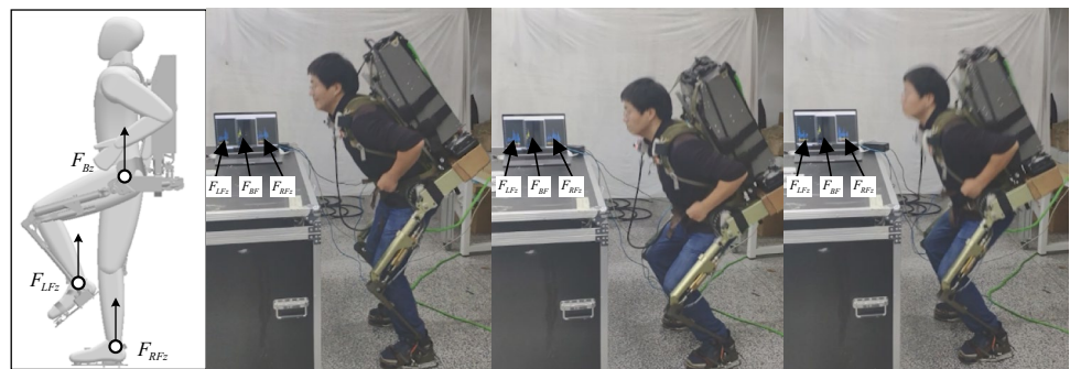
Fig. 11 Exoskeleton non-powered, follow-up, and active assistance experiments
