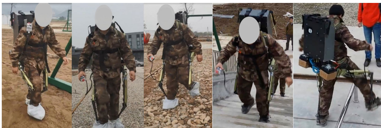
Fig. 13 Active power-assist experiments in challenging terrains
