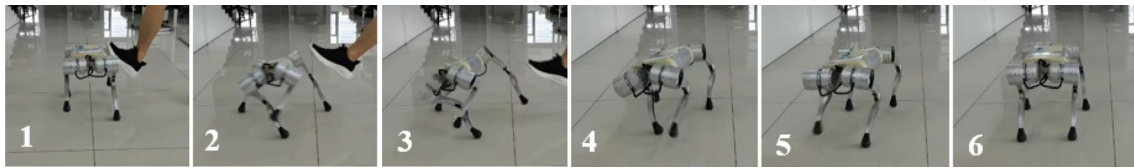
Fig. 9 The robot loses balance after being subjected to a lateral impact, and quickly recovers stable by changing step frequency
