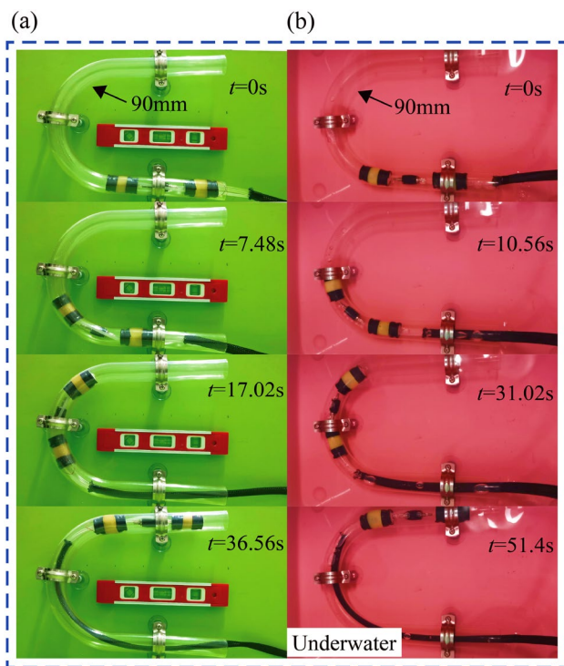
Fig. 15 motion experiment in an unstructured environment a motion in a U-pipe, b motion in a U-pipe filled with water
