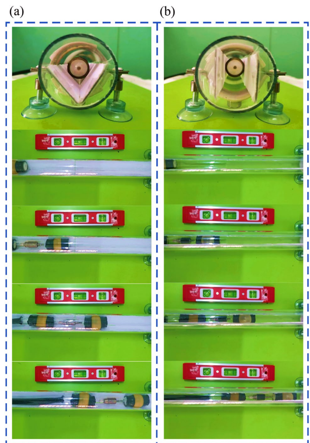
Fig. 16 non-round pipe experiments: a fan-shaped pipe, b oval pipe
