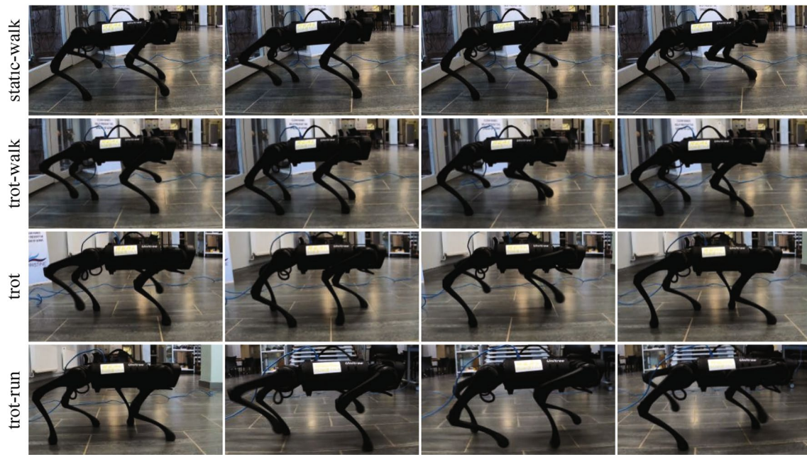
Fig. 11 Snapshots of the robot running with multiple gaits. From top to bottom, the speed of each gait increases respectively
