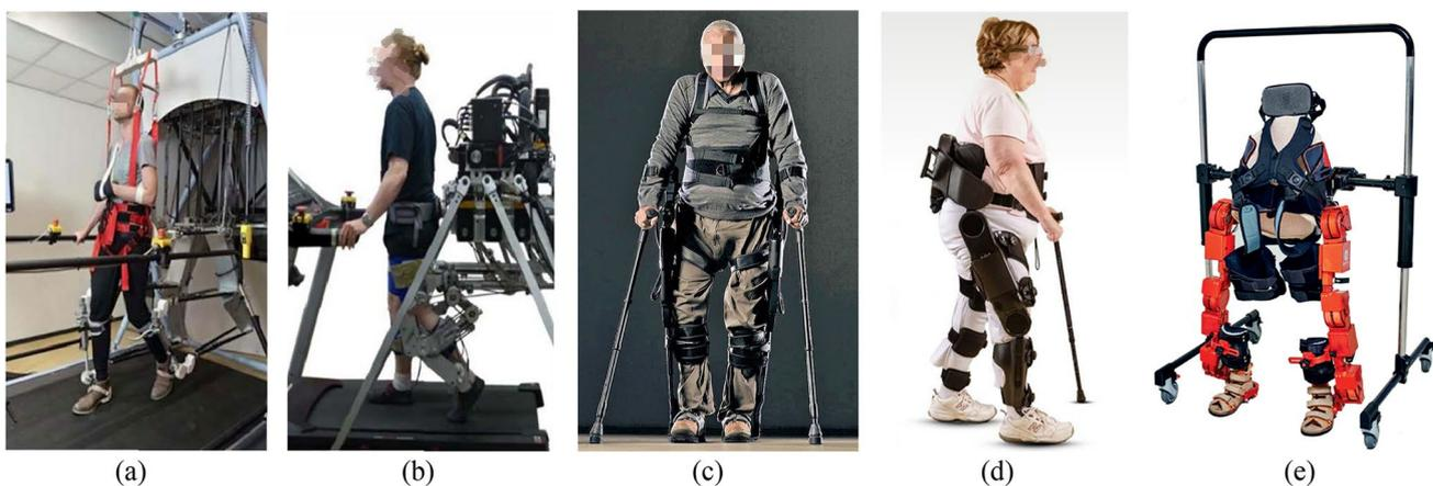
**Fig. 10** Representative of medical rehabilitation LEEX: **a** LOPES II [130] **b** ALEX III [131] **c** Ekso-GT [132] **d** Indego [133] **e** Atlas 2030 [134]
