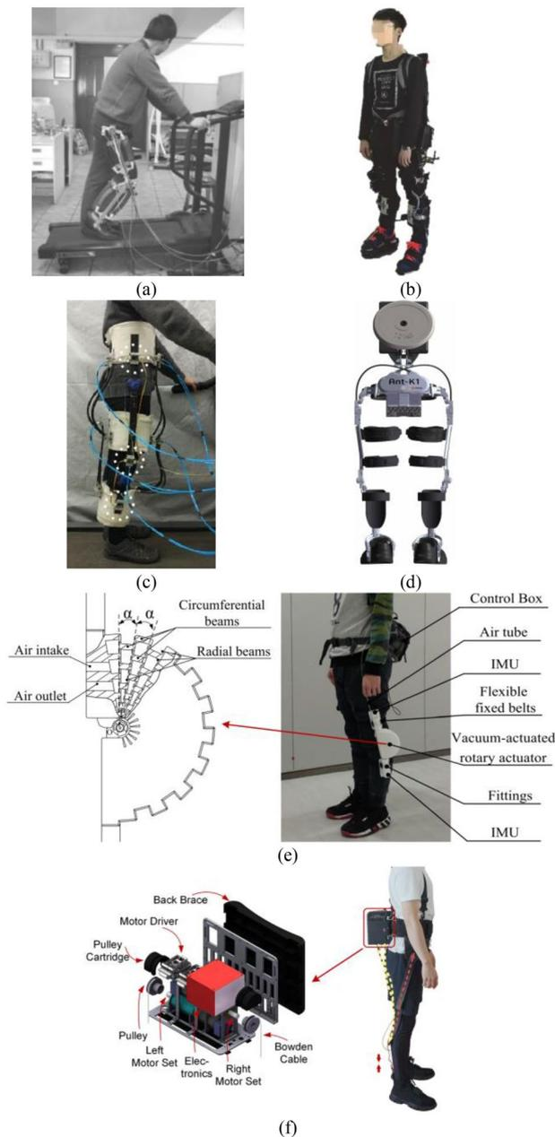
**Fig. 7** Representative CLEEX in China: **a** Pneumatic muscles exoskeleton, Harbin Engineering University [111] **b** rope driven exoskeleton, the SIAT of the CAS [112] **c** flexible exoskeleton, Southeast University [114] **d** Ant-K1, Kenqing Technology [115] **e** soft knee exoskeleton, Beijing Institute of Technology [116] **f** exosuit, SIACAS [117]
