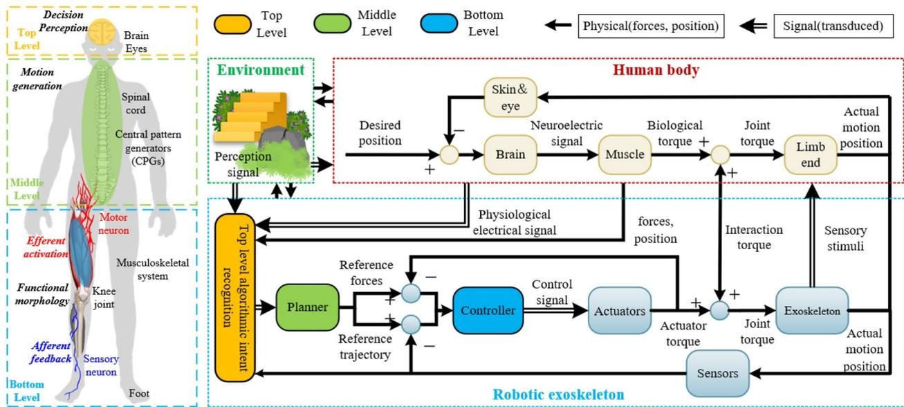
Fig. 16 Control diagram of the human–exoskeleton environment-coupled system
