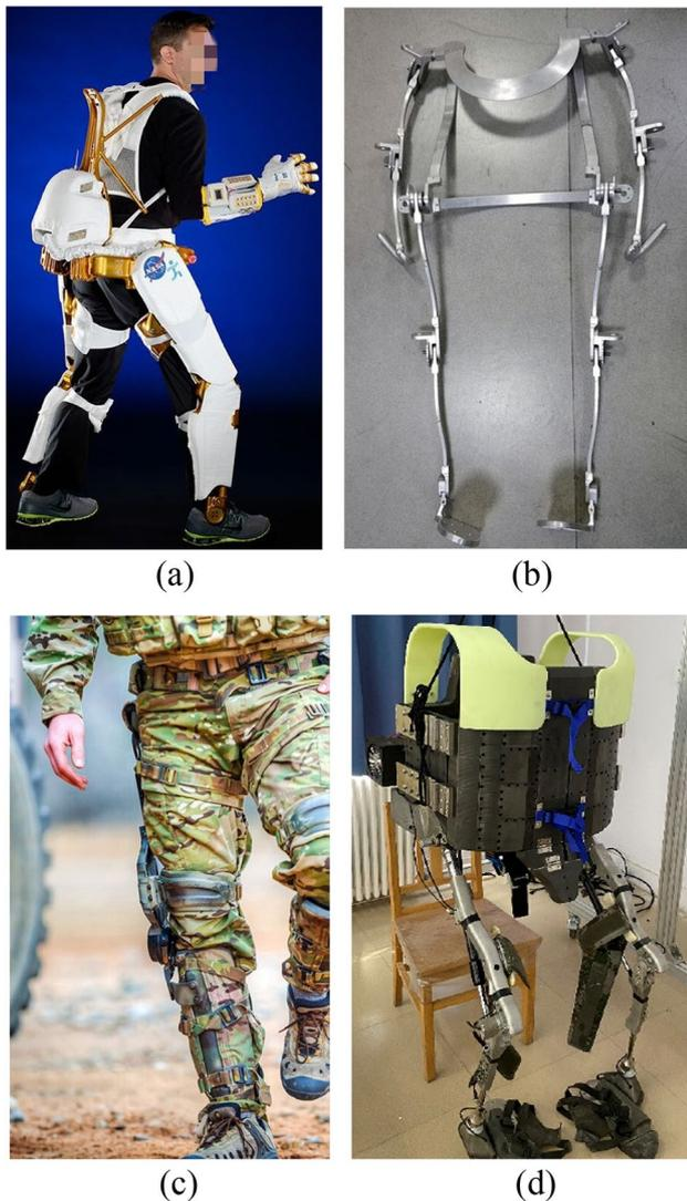
**Fig. 11** Representative of special functional classification of LEEEX: **a** X1, NASA [136] **b** 2nd joint-assisted exoskeleton, UESTC [138] **c** Prowler, Revision Military [139] **d** fast neutron shielding suit with human exoskeleton, LZU [140]
