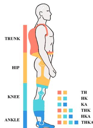
**Fig. 3** Classification of multi-joint lower extremity exoskeletons *TH* trunk–hip, *hk* hip–knee, *KA* knee–ankle, *THK* trunk–hip–knee, *HKA* hip–knee–ankle, *THKA* trunk–hip–knee–ankle
