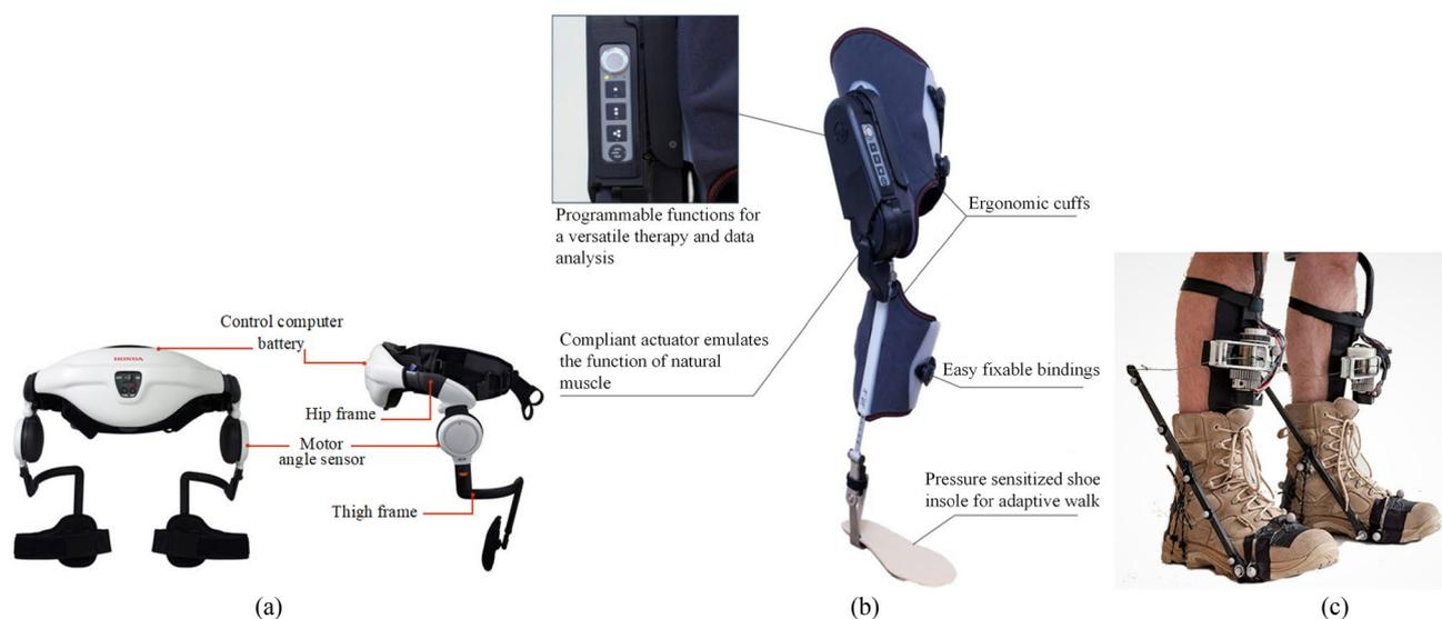
**Fig. 2** Single joint lower extremity exoskeleton systems. **a** Walking Assist [58] **b** MAK [60] **c** Autonomous leg [62]
