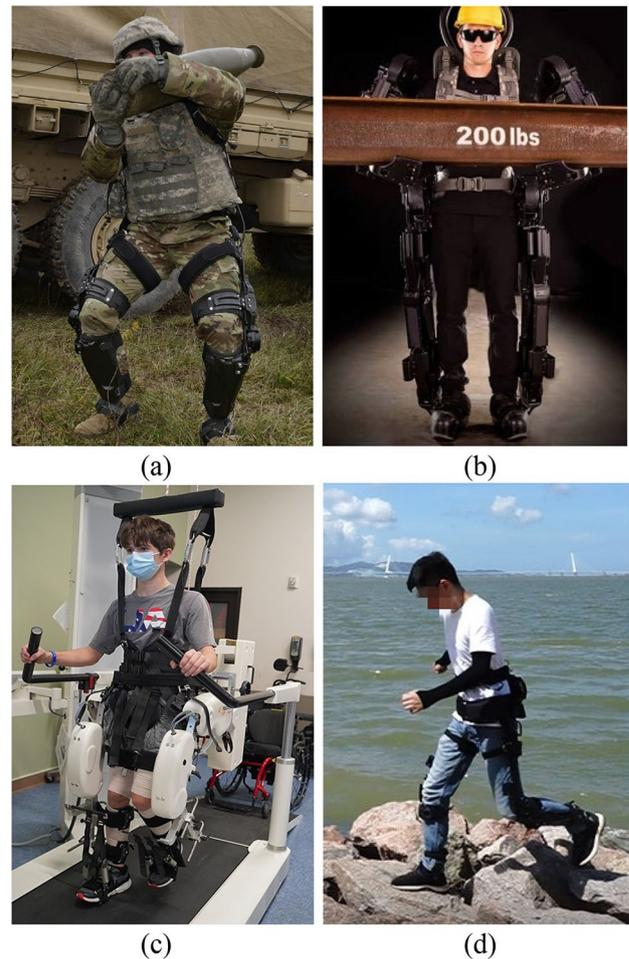
**Fig. 12** LEEEX in different industries: **a** military field [141], **b** industrial field [142], **c** medical field [143], and **d** consumer field [146]
