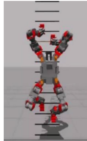
Fig. 6 Verification of the new proposed ladder climbing gait in simulation
