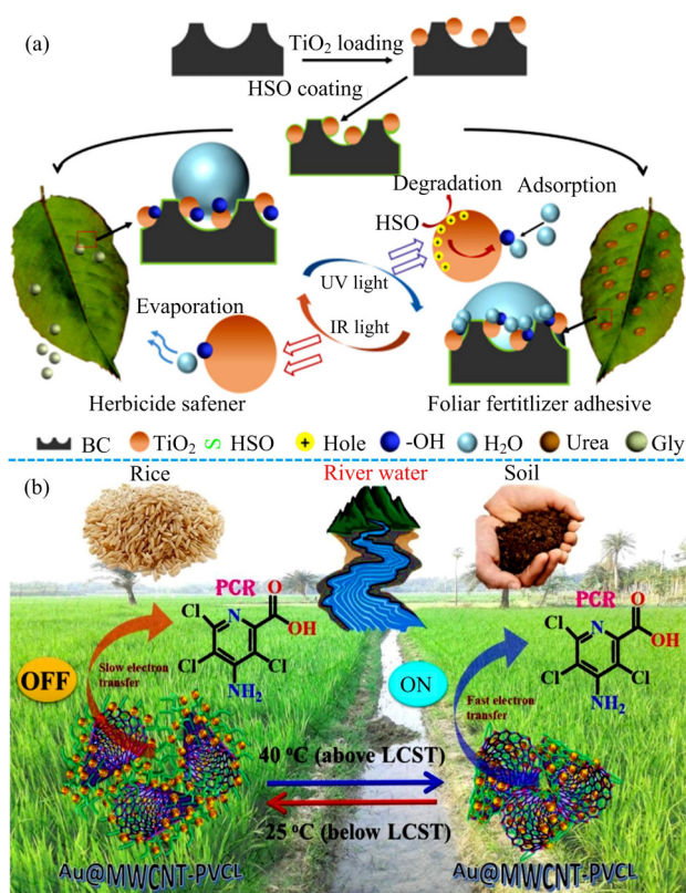
Fig. 15 (a) The light-responsive smart surface used for herbicide safener or foliar fertilizer adhesive, hydrophilic LHNS can improved the adhesion of foliar fertilizer; hydrophobic LHNS can prevent the adsorption of the amount of water and used as a glycine safener [169] . (b) The smart surface upon temperature for PCR detection, the hydrophilic surface of PVCL at 25 °C prevent the PCR pass over in “OFF” state, while the switched hydrophobic surface at 40 °C upgrade PCR oxidation in “ON” state [170] .
