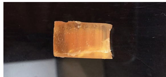
Fig. 8 The adhesive material adhering on glass wall.
