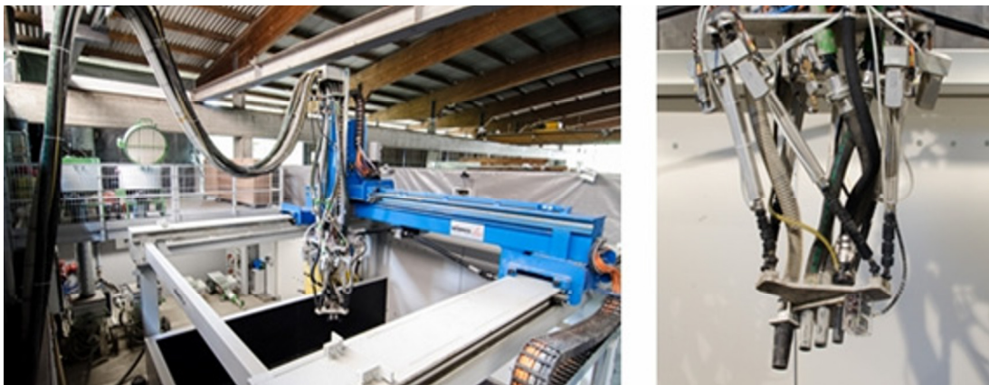
Fig. 5 Automated multi-nozzle machine for the reproducible production of graded concrete components. The two spraying nozzles are applied to one spraying head to facilitate continuous processing [28] .
