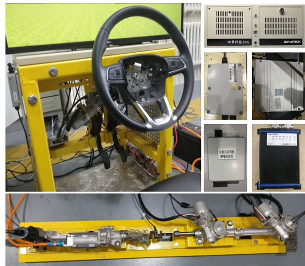
Fig. 11 The HIL bench
