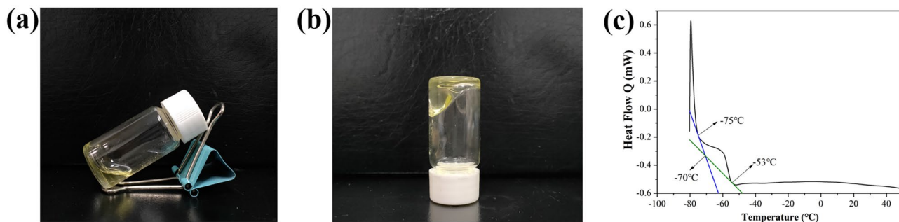
Fig. 3 Inclined a and inverted b views of the CLP-boroxine in vial, and DSC curves c of CLP-boroxine at -80\text{ }^{\circ}\text{C} – 50\text{ }^{\circ}\text{C}
