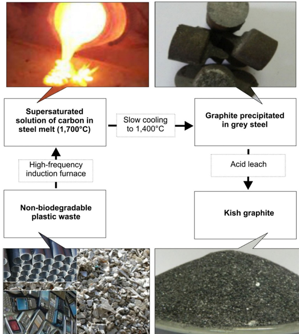
Fig. 13 Procedure for the generation of kish graphite. Reproduced with permission [183] Copyright © 2019 Springer-Verlag GmbH Germany
