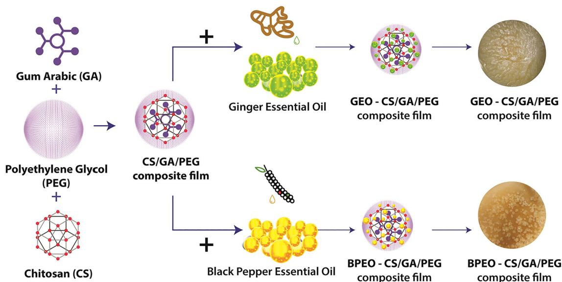
Fig. 1 Schematic illustration of the preparation of CS/GA/PEG composite film with and without BPEO and GEO
