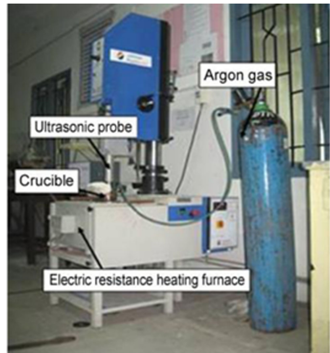
Fig. 1 (a) Experimental setup for fabricating nanocomposites
