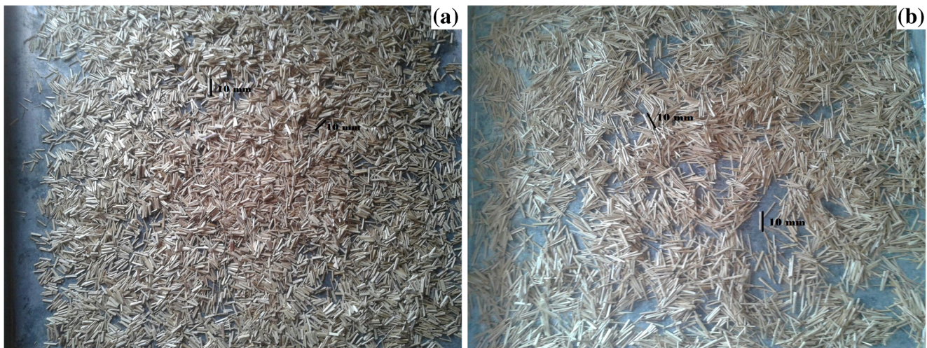
Fig. 1 a Before chemical treatment of bagasse fiber. b After chemical treatment of bagasse fiber
