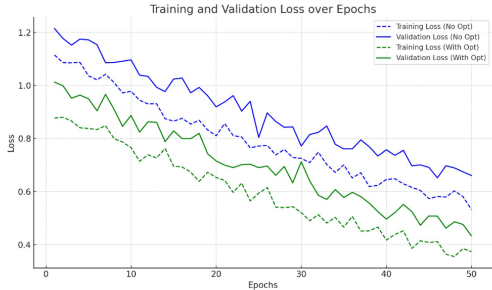
Fig. 4 Training and validation loss over epochs for both models (LGBM without optimization and LGBM with Locust Swarm Optimization)
