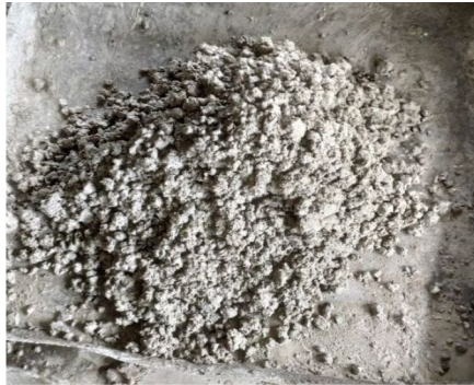
Fig. 8 Fresh geopolymer concrete
