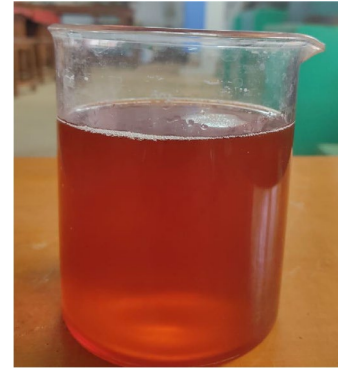
Fig. 6 ViscoCrete: PCE-based chemical admixture
