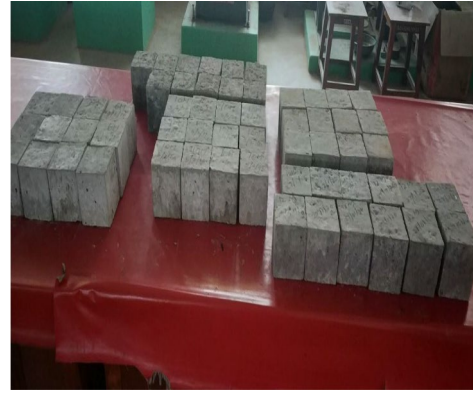
Fig. 10 Cubes under ambient curing
