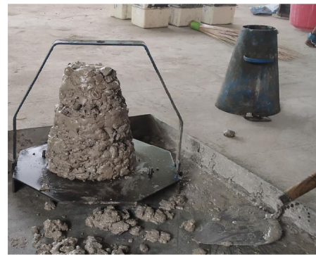
Fig. 11 Slump cone test on geopolymer concrete
