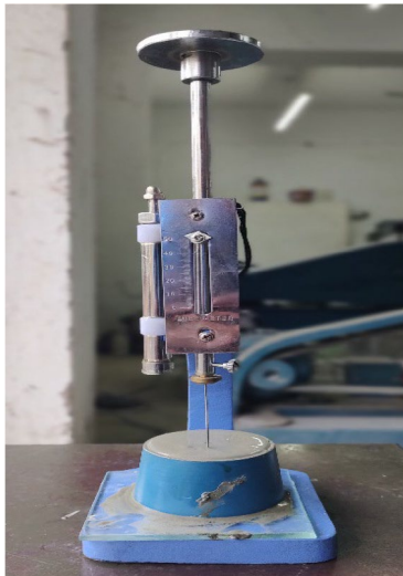
Fig. 12 Initial setting time test
