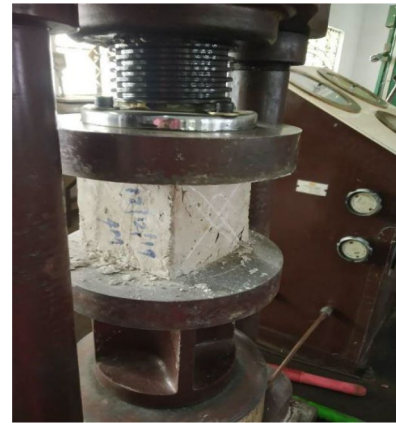
Fig. 14 Compression test on geopolymer concrete cube
