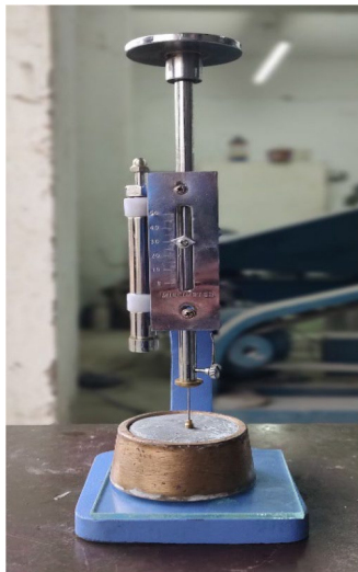
Fig. 13 Final setting time test
