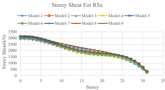
Fig. 26 Storey shear in X-direction
