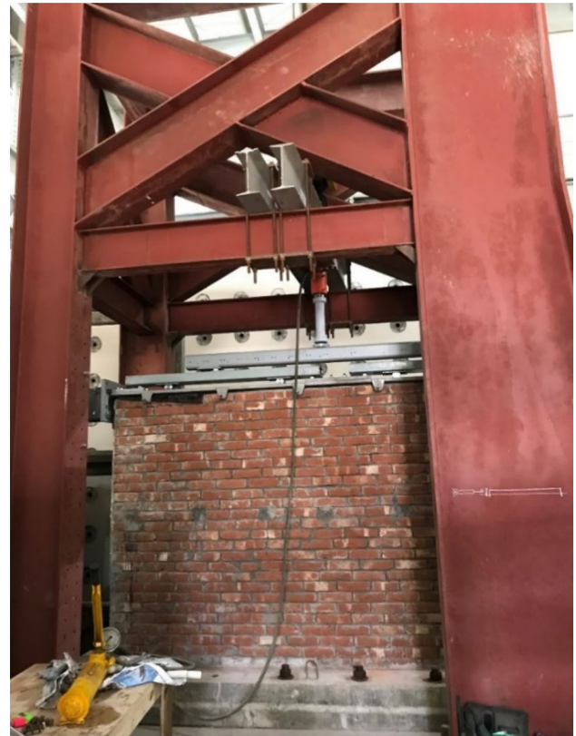
Fig. 14 Hydraulic jack over wall
