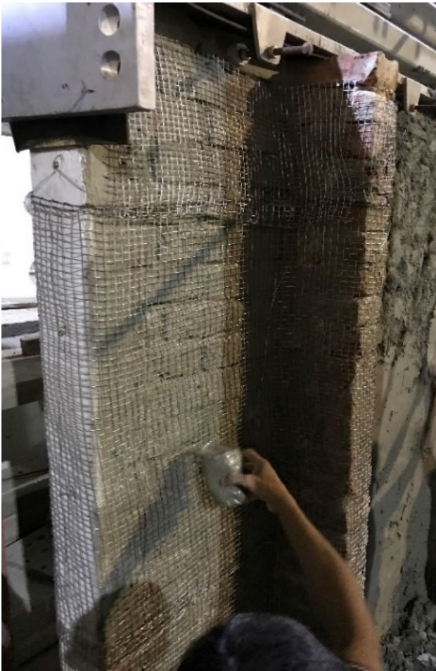
Fig. 8 Wire mesh confinement processing
