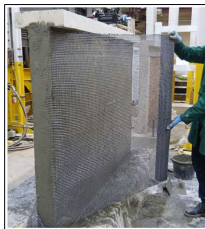
Fig. 10 TRM wrapped around MIW Koutas and Bournas (2019)
