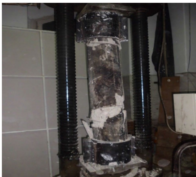
Fig. 6 Column failure mode
