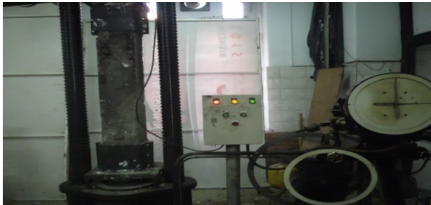
Fig. 5 Column test set-up
