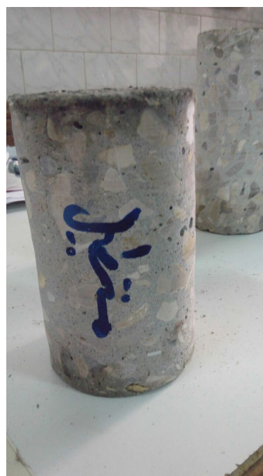
Fig. 7 Core specimen cut from a rectangular column
