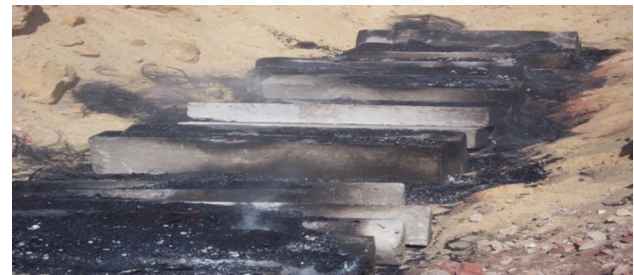
Fig. 2 Column samples subjected to fire
