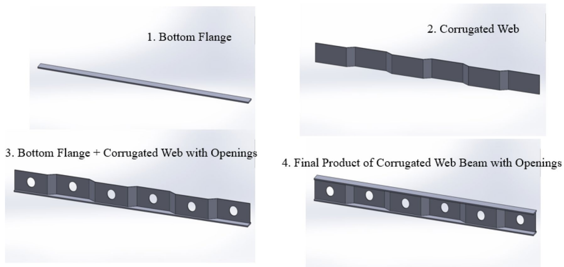
Fig. 1 Step by step fabrication procedure of steel corrugated beam with web openings
