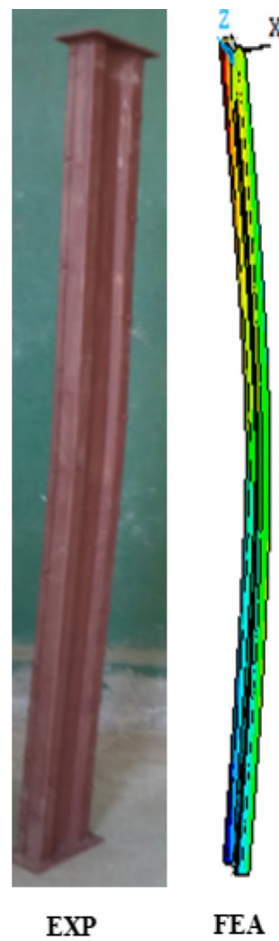
Fig. 14 Comparison of experimental and FEA-deformed shape for specimen BC40L2240
