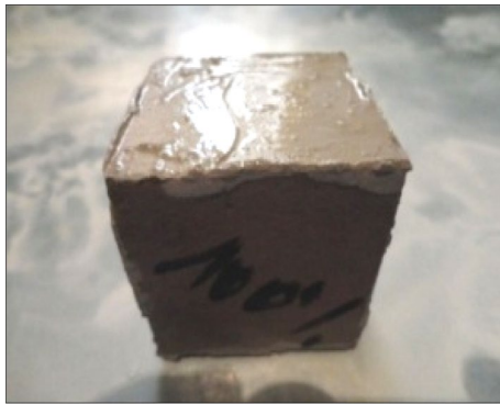
Fig. 4 Composite mortar WPLAX coated with epoxy resin prior to sorptivity test and immersion in 5% NaCl solution
