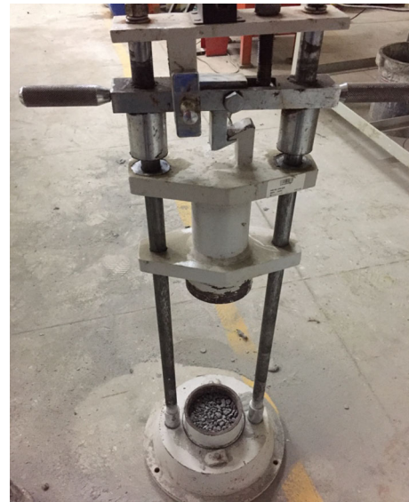
Fig. 6 Test setup for impact strength of lightweight aggregate and conventional aggregate
