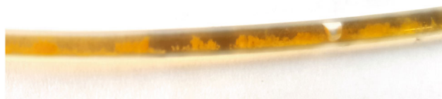
Fig. 11 Precipitation of the ferrioxalate actinometer after too long irradiation in a FEP capillary
