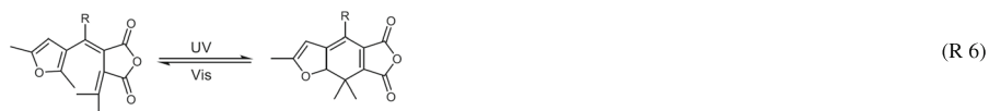
Fig. 3 Reaction equations for three of the most common actinometer systems: ferrioxalate, Reinecke's salt and Aberchrome 540
