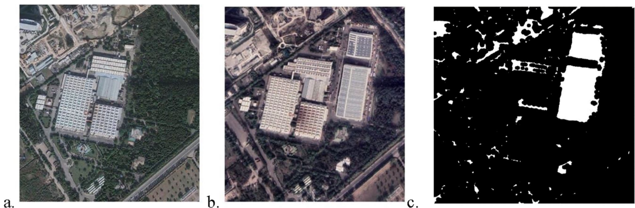
Fig. 8 Change map generated using binary edge detection techniques and ML algo on temporal TripletSat data 2015 and 2018. a T0, pre-image; b post-image; c change map (white pixel, change; black pixel, no change)
