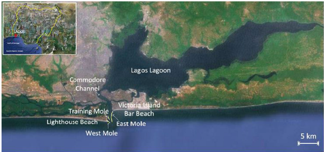
Fig. 2 A section of the Lagos shoreline highlighting the west and east mole constructions source: [34]
