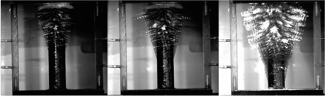
Fig. 5 Three high-speed video frames of explosively driven CFC at 15, 17, and 21 \mu s
