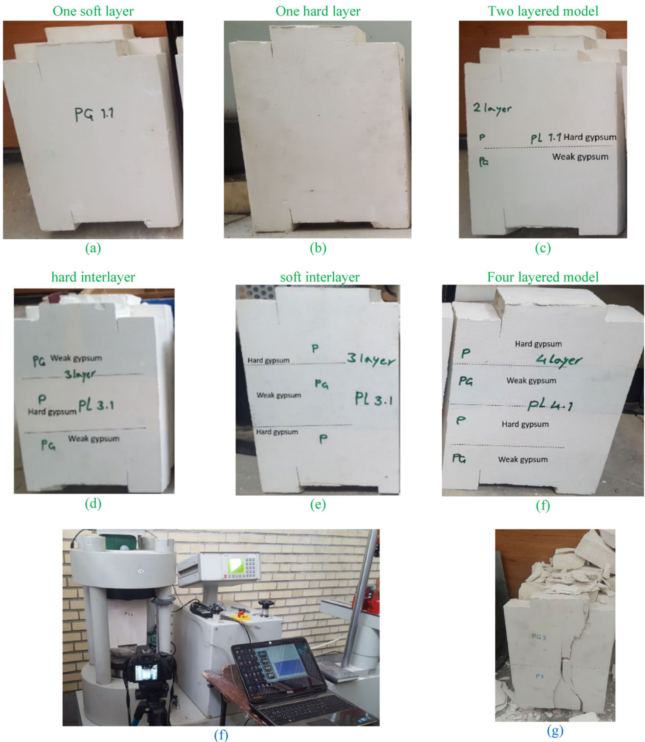
Fig. 3 Depict physical samples as follows: a a single soft layer, b a single hard layer, c a two-layered model, d a three-layered model with a hard interlayer, and e a three-layered model with a soft interlayer, f punch shear test device, g three similar samples tested from each layer configuration
