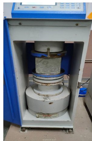
Fig. 1 Arrangement for compressive strength test
