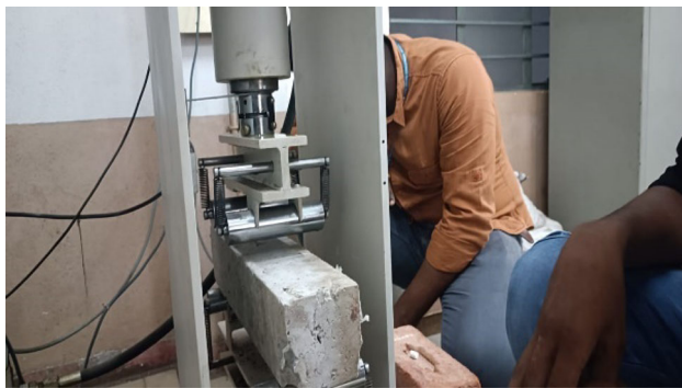
Fig. 2 Arrangements for flexural strength test
