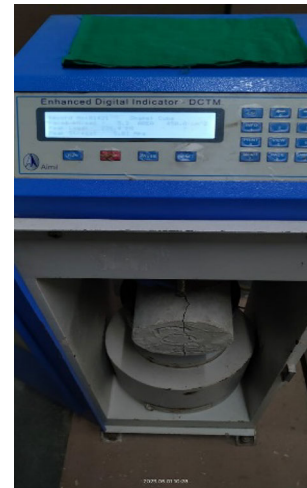
Fig. 3 Arrangement for split tensile strength test
