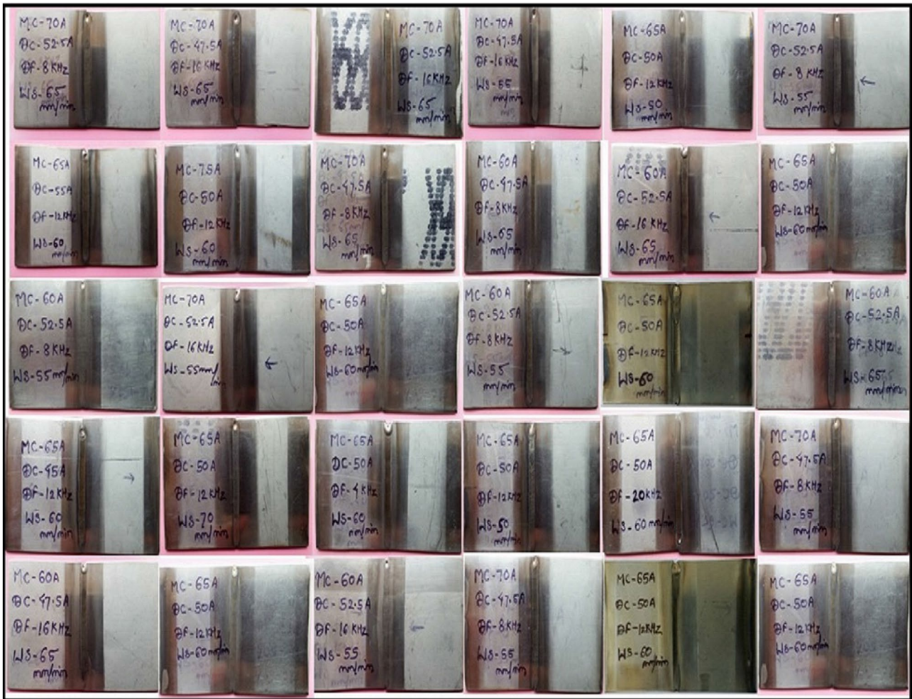
Fig. 4 GTCA welded joints of Inconel 718 alloy
