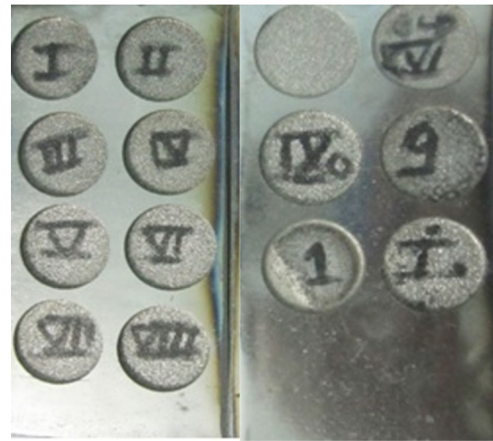
Fig. 4 Machined workpiece by copper tool
